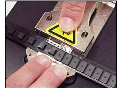
To trim the opposite side of the spliced carrier tape, position the reel stand on the other side of the tape splicer. Repeat Steps 6 and 7.
